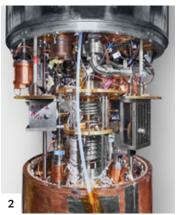
SCIENTISTS attach sensors to the experiment insert (1). Above the insert's copper-plated cavity is a liquid-helium reservoir surrounding electronics (2).
